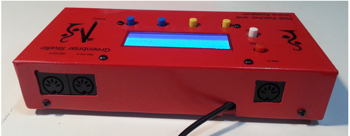
Old Model Midi Assigner New Model has Two Midi Ins and longer case
